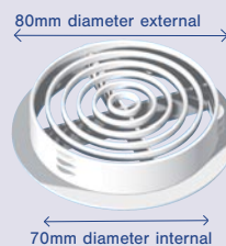
10mm Air Gap = 200mm centres 25mm Air Gap = 85mm centres
